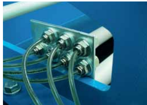
Zentrales Schmiersystem / Central lubrication system
