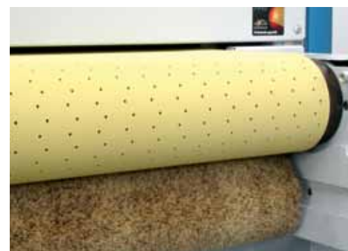
Gurtreinigungsbürste / Cleaning brush for conveyor belt
