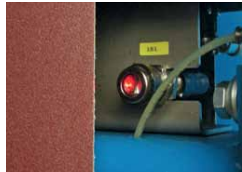
Fotozelle / Photo-optic sensor
